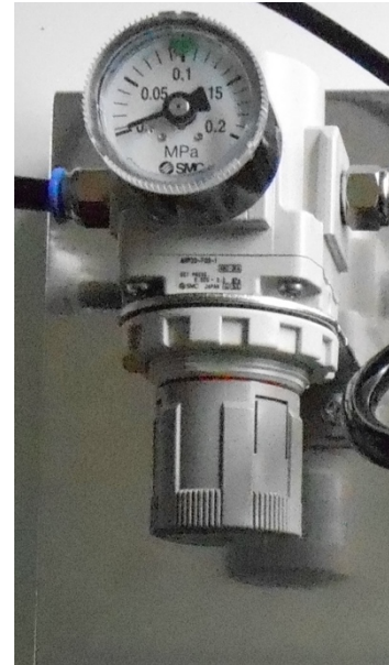
Manual air pressure regulator
