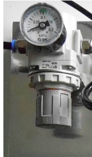
Manual air pressure regulator
