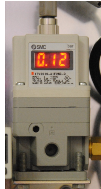
Automatic air pressure regulator
