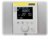
Controller mounted on kiln door and removable for comfortable operation
