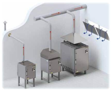
Example for exhaust air connection when bypass connector or exhaust hood are used
