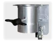
Semi-automatic air inlet flap for residual drying in chamber kilns up to 300 liters. The flap closes automatically at a set temperature and does not have to be closed manually after the drying phase.
