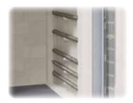
Three-sided heating with heating elements on support tubes (N 500 E)
