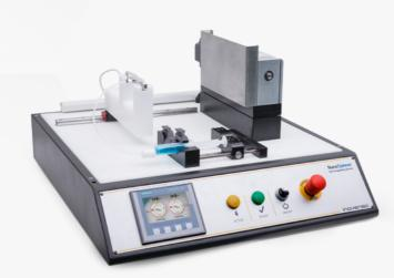
It is possible to apply high voltage with precision as well as adjust the flow rate and the distance between the needle and collector.
