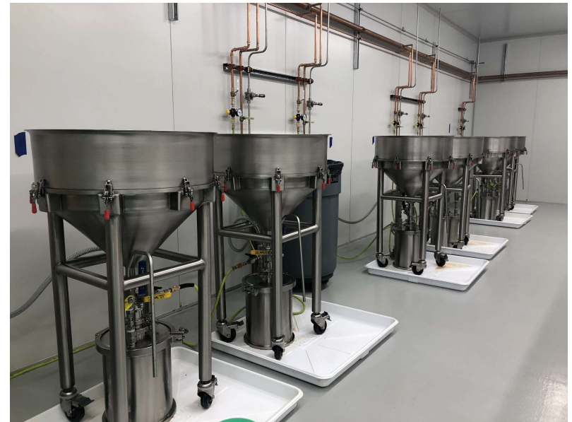
DrainDroyd Vacuum Filtration Reservoir Volume 150 L
