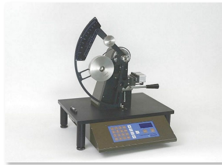
The Model DE-1600-CF Digital Elmendorf Tear Tester with 200 gram Framework Pendulum and 1600 gram Add-Weight for a 1600 gram Tear measurement capacity. Includes Pneumatic Sample Clamps and Integral Sample Cutting Knife
