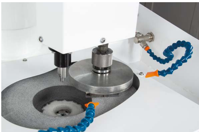
Prepolishing of large raw samples.
