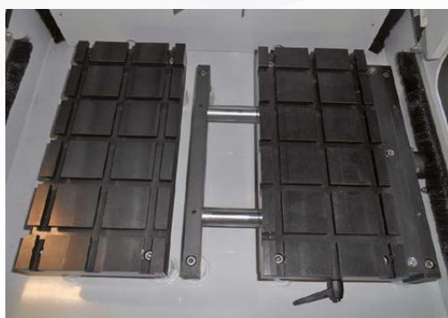
Transversal table X axis 120 mm stroke
