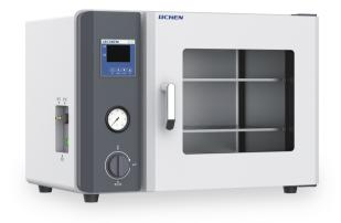
DZF series vacuum drying oven is specially designed for drying heat-sensitive, easy to decompose and easy to oxidise substances, when working, it can keep a certain degree of vacuum in the working chamber, and it can be filled with inert gas to the inside, so that the items in the box, especially some items with complex composition, can be dried quickly, and it adopts the intelligent digital temperature regulator for setting, displaying and controlling the temperature.
