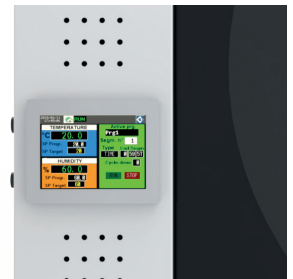
The revoFACE programmer is designed for cycle testing.
