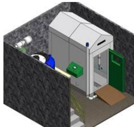
660 cu. ft. walk-in corrosion chamber designed in accordance to ASTM B117 and ISO 9227
