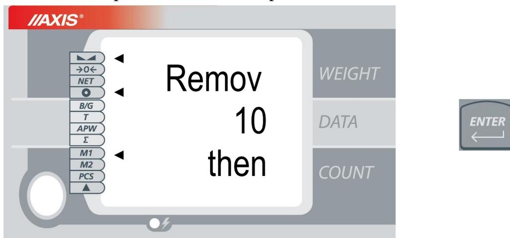
3. *Remove 10 then* press **Enter** communicate will appear. Remove one or more details from the portion.
