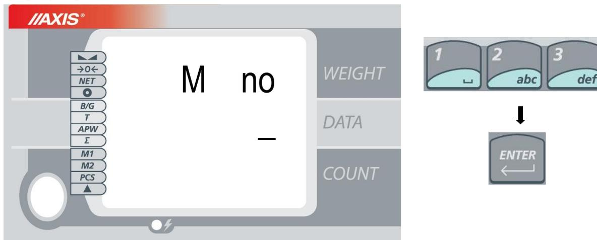
On upper section display *M no* sign shows up and on the middle section a field to inscribe record number ( from 1 to 1000). Inscribe the number using numerical keys and confirm by pressing **ENTER**.
