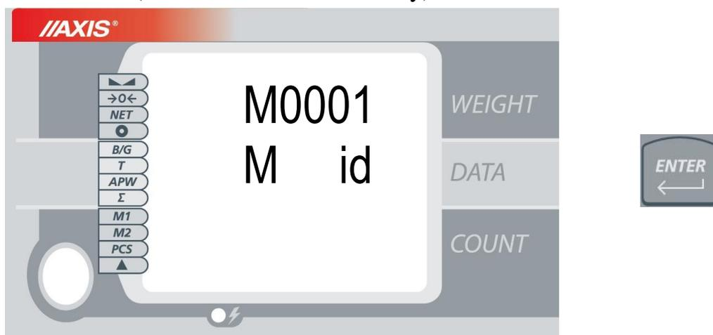
To speed up options displaying user can press  $\Sigma+$  ,  $\Sigma-$  or  $\rightarrow 0 \leftarrow$  button.
