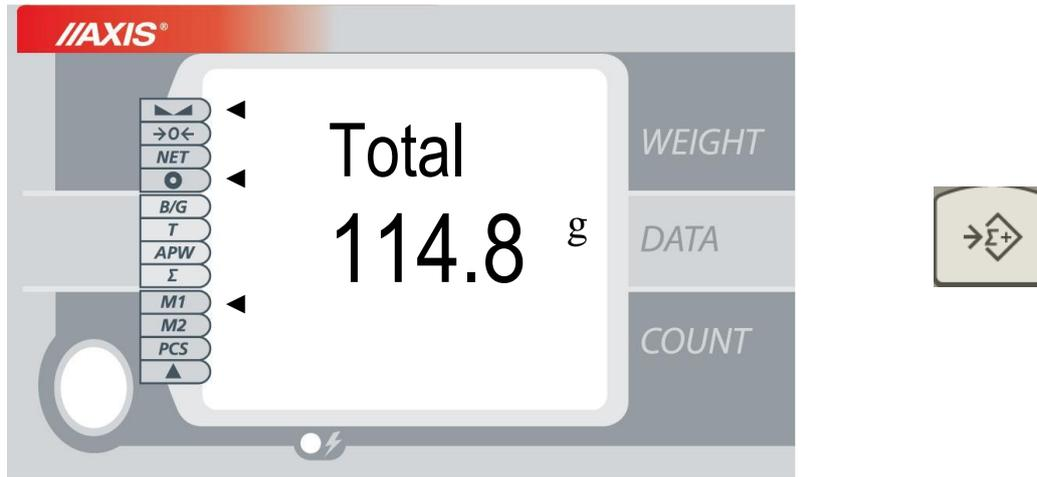
1. Put weighted element on the pan and press  $\rightarrow \Sigma+$  button. Contents of this register have been showed temporary in middle section display, the upper section displays *Total* sign.
