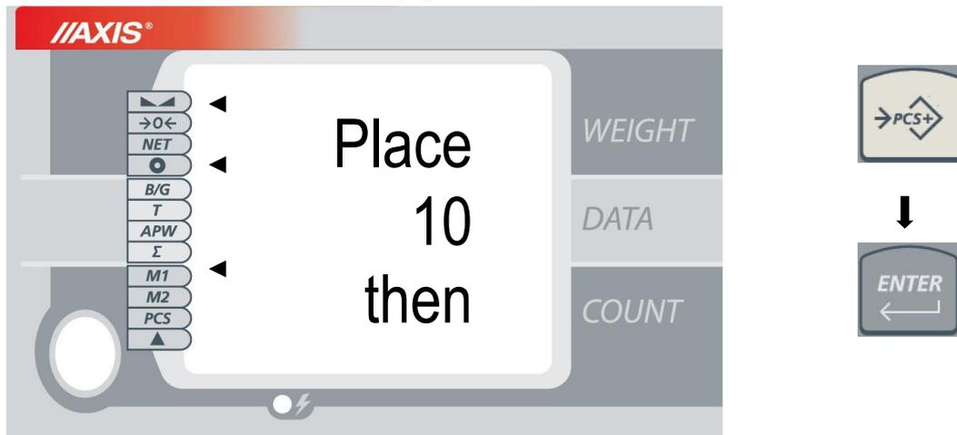
3. *Place 10 then press Enter* communicate will appear. If the quantified sample consists 10 pieces press *ENTER*. If amount of detail is other write correct value by using numeric keys and press *ENTER*.
