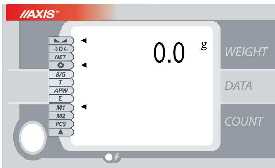
Scale display is divided into three sections: **WEIGHT** - upper, **DATA** - middle and **COUNT** - lower. Each of these sections has its own measurement indication and information indicators that complement main information or describe scale state. Indicator is active when there is a ◀ mark next to it. On above screen ◀, ● and *M1* indicator is active.
