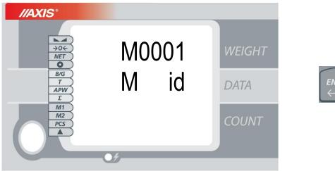
To speed up options displaying user can press  $\Sigma$ +,  $\Sigma$ - or  $\rightarrow 0 \leftarrow$  button. To choose option press *ENTER* key.
