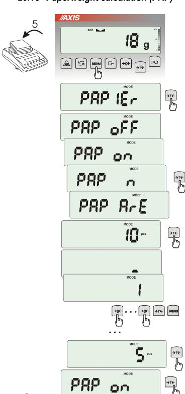
This function enables to calculate paperweight of 1m<sup>2</sup> of paper basing on samples of known area. For quick access, the function is accessible directly by pressing *MENU* key.
