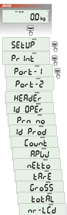
Function is used for printing additional information stored in scale memory, weighed product identification data and scale operator id. That information is inscribed using scale keys or scanner. After entering selected port (scale can have two ports) user may activate printout positions:
