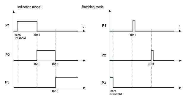
In *Batching* mode on P1 (thr I) and P2 (thr II) outputs short-circuit impulses appears for time of 0,5s. On P3 (zero) output short-circuit state appears when indication does not exceed threshold value signalling zero load.
