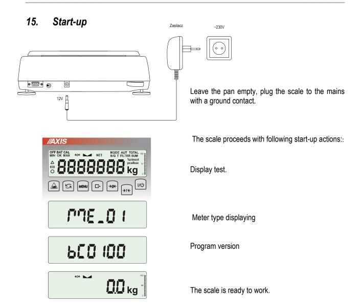
**Attention:** UnLOAd communicate means that the scale is loaded or transportation security elements situated under the pan has not been removed.
