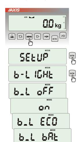
The function is used for choosing the work mode of scale display backlight:
