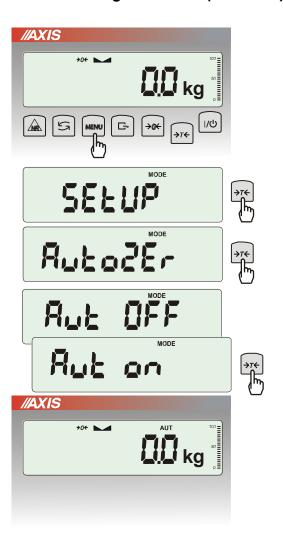
When the function is activated, the scale automatically ensures stable zero indication if the pan is empty or if zero indication was acquired by pressing  $\rightarrow T \leftarrow$  key.
