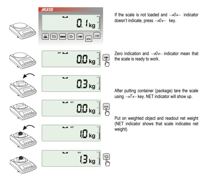
In order to readout gross weight press  $\leftrightarrow$  key (B/G indicator shows that scale indicates gross weight). Press again  $\leftrightarrow$  key in order to come back to net indications.
