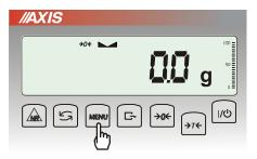
Before measurement scale should be tared. Function has following options:
