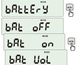
*bAttErY* function allows switching on or off charging accumulators during work with feeder and checking their power level.
