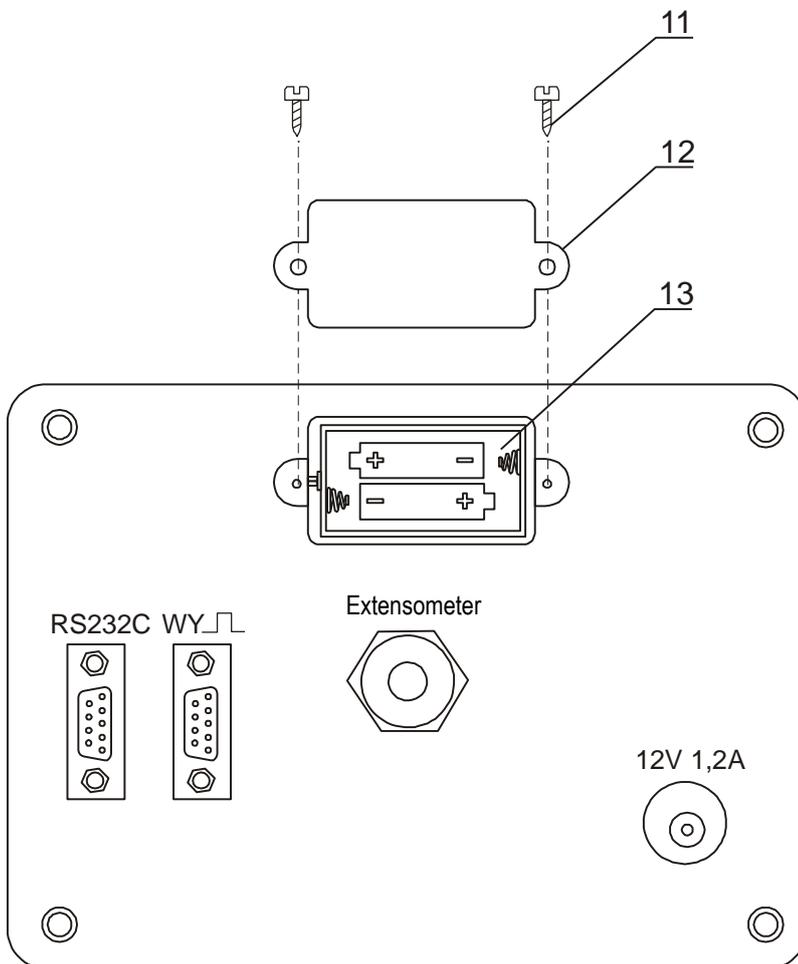
1. Remove screws 11 holding plate 12, remove the plate.
