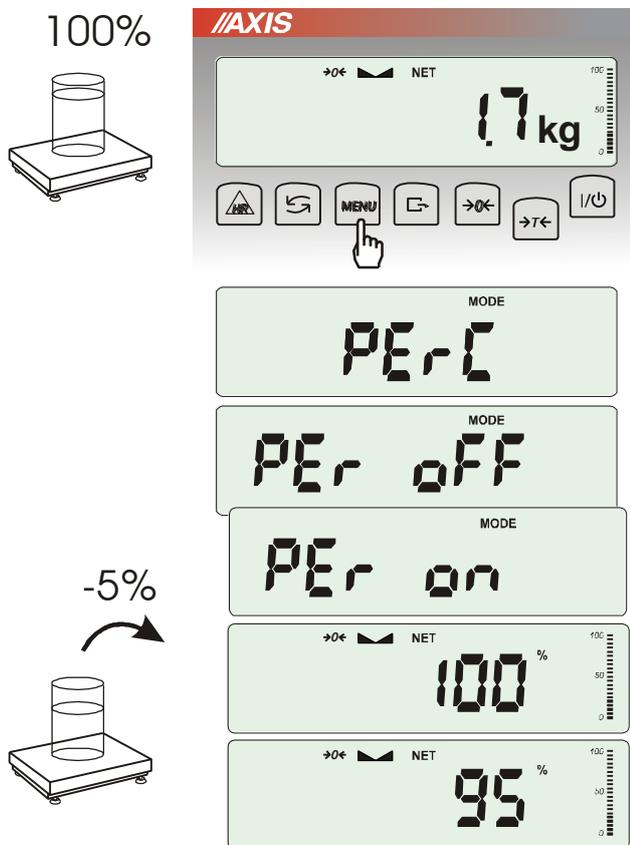
This function allows displaying weighing result in percents.
