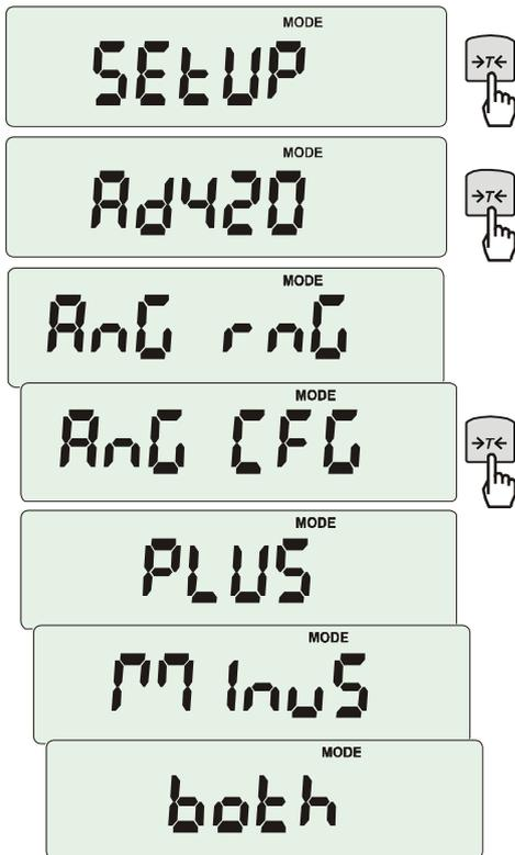
This option enables to set-up analog out (4-20mA or 0-10V) working method used e.g. in PLC regulators:
