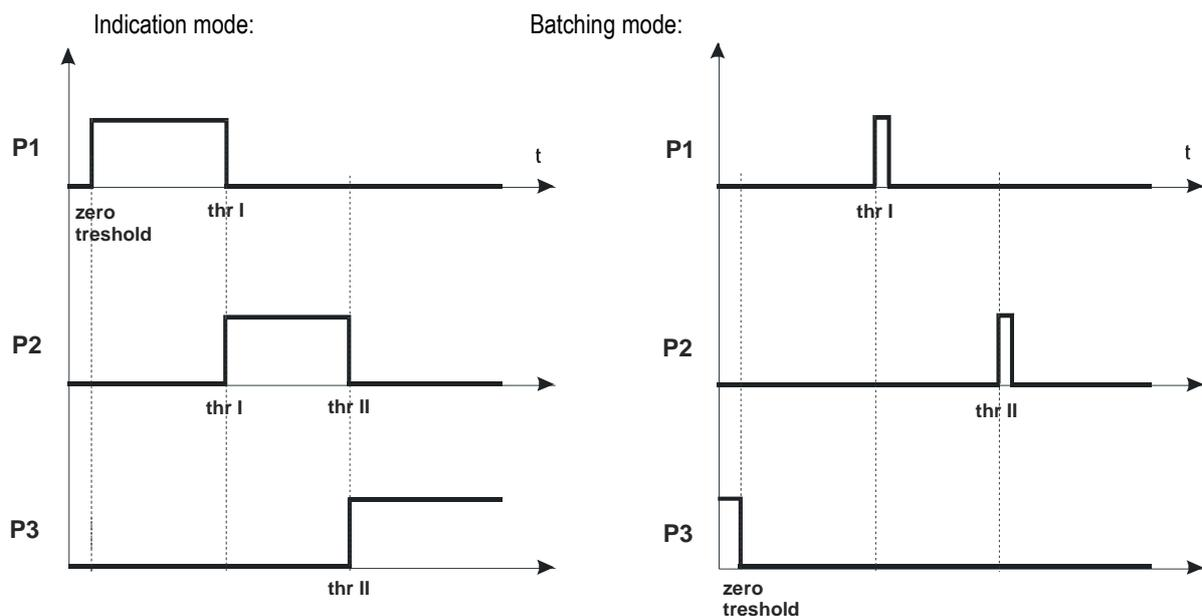
In *Batching mode* on P1 (thr I) and P2 (thr II) outputs short-circuit impulses appears for time of 0,5s. On P3 (zero) output short-circuit state appears when indication does not exceed threshold value signalling zero load.
