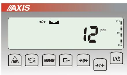
During standard weighing ↻ key is used to switch between net and gross indication.
