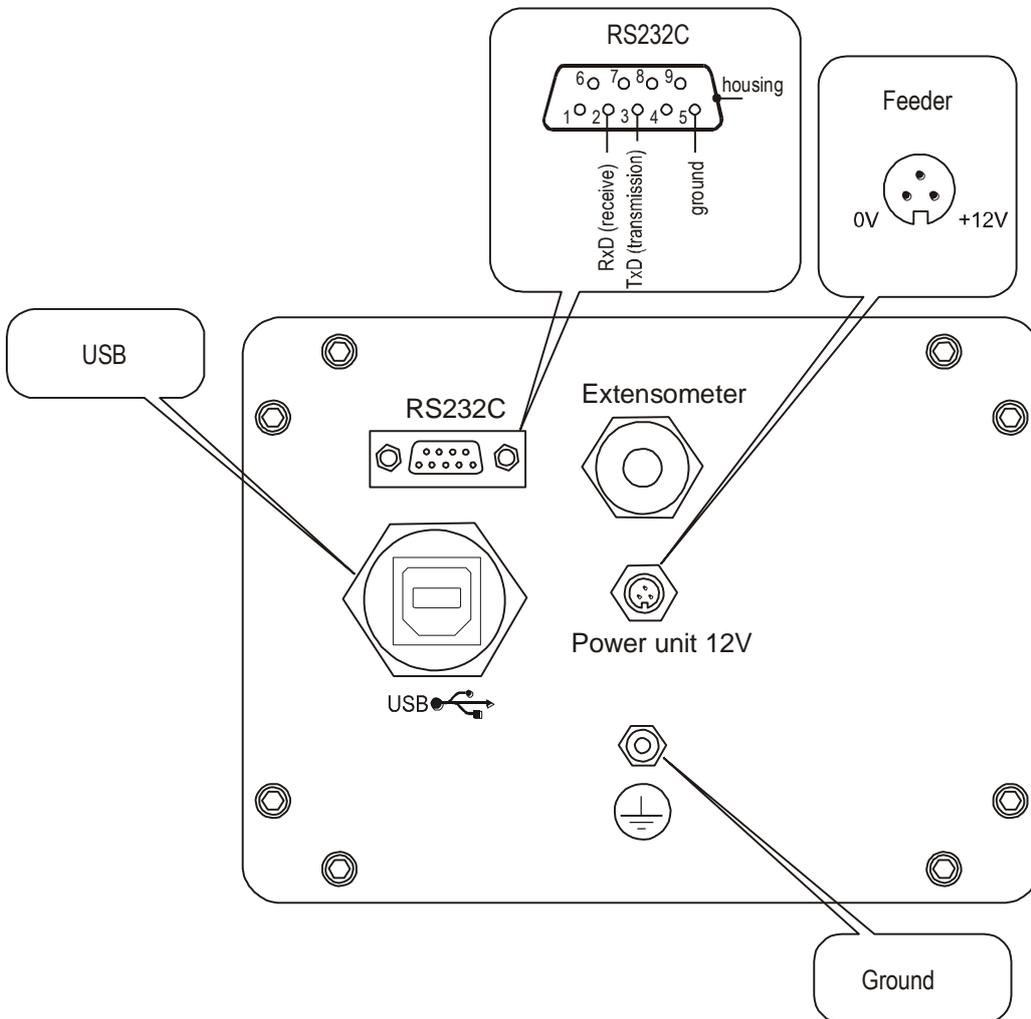
Separate ground connection (scales in stainless steel version) must be connected using additional conductor.
