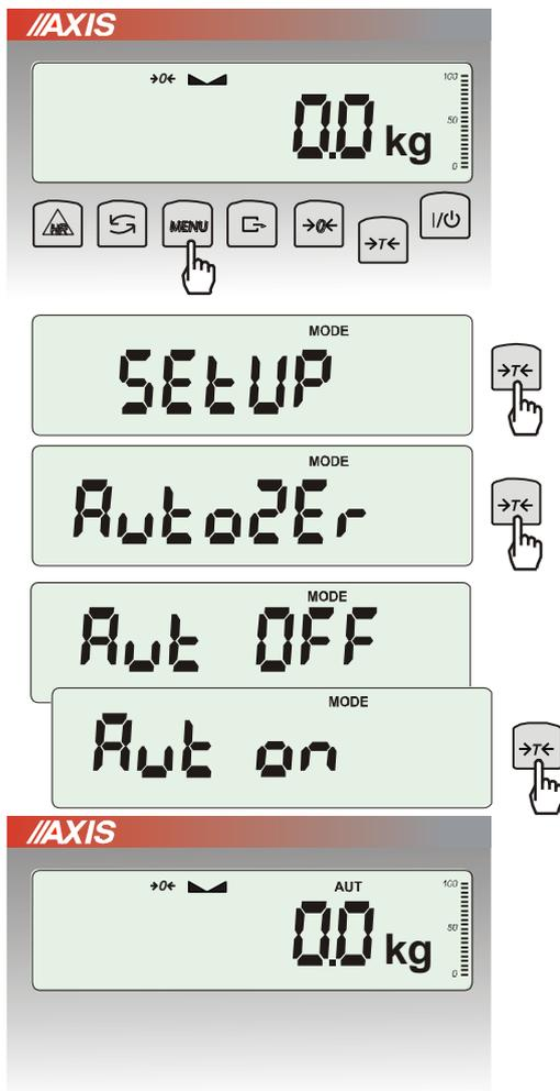
When the function is activated, the scale automatically ensures stable zero indication if the pan is empty or if zero indication was acquired by pressing →T← key.
