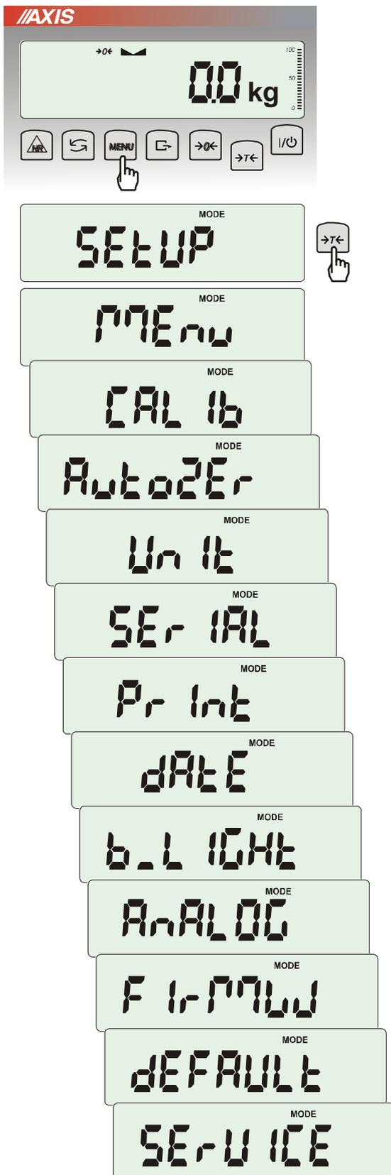
SEtUP contains all options used for setting scale work mode:
