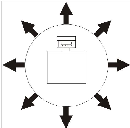
The workplace should be carefully chosen in order to keep to minimum influence of external factors that can disturb balance work. Proper temperature and work space is crucial. Balance should stand on stable foundation made of non-magnetic impact material.
