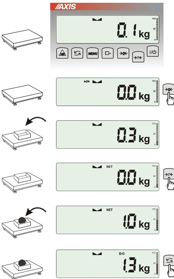
If the scale is not loaded and  $\rightarrow 0 \leftarrow$  indicator doesn't indicate, press  $\rightarrow 0 \leftarrow$  key.
