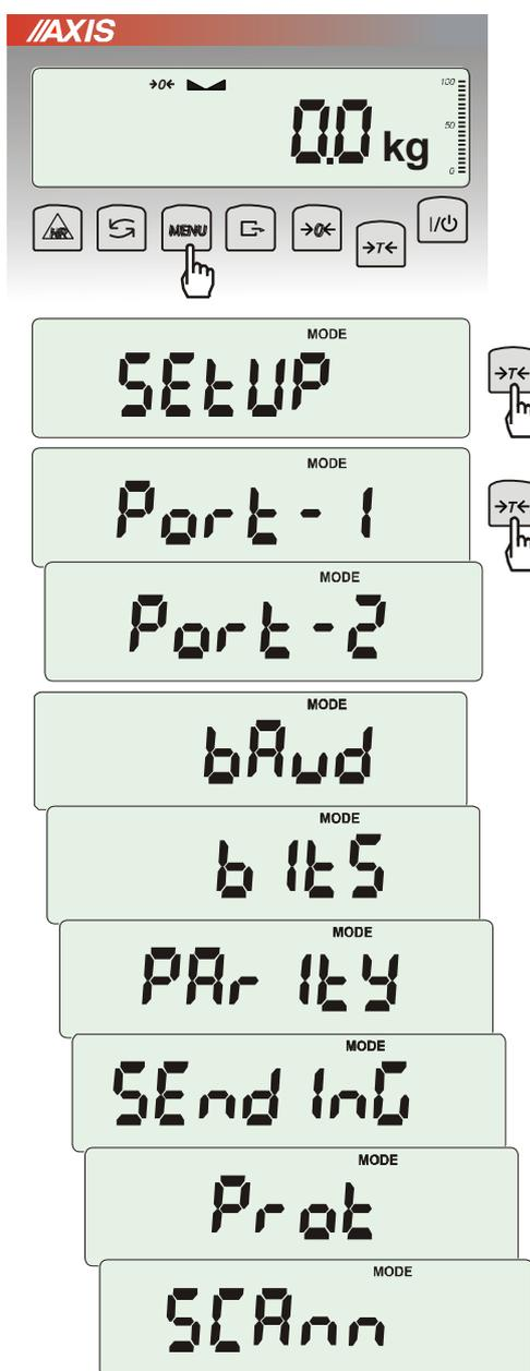
The function allows setting independently communication parameters of both of serial ports *Port-1* and *Port-2* (executed in RS232C, RS485, USB or LAN standard):
