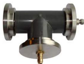
end plugs are mounted on the plastic pipe T-fitting
