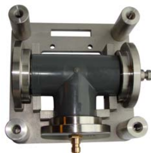
the end plugs and plastic fitting are placed in the containment cage
