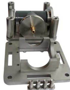
the lid of the containment cage is ready to be fixed and pressure testing may commence
